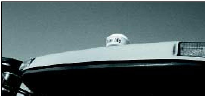
Figure 2.6 Sample Antenna Mount above Cab
