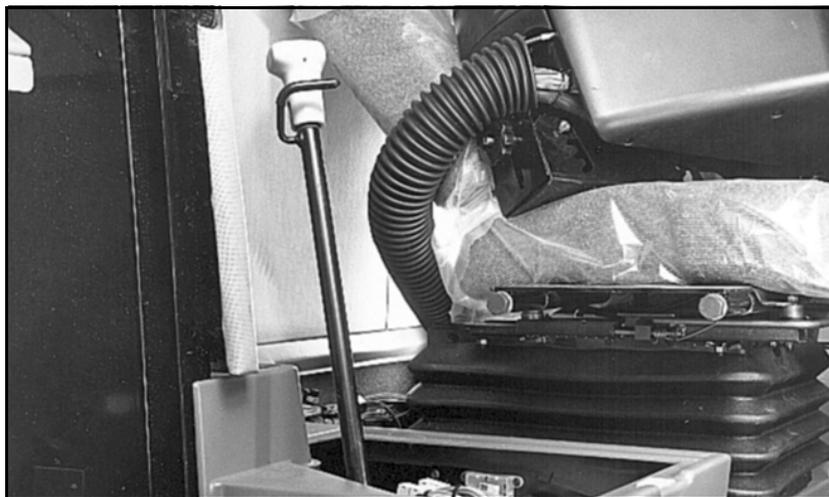
Figure 2.20 CASE-IH Cable Connection Under Seat Console
