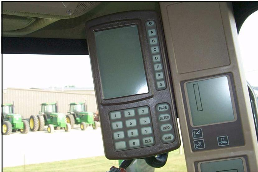
Figure 2.23 GreenStar Display on Right-Hand Cab Post
